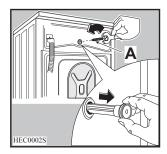
Unscrew and remove the two large rear bolts **B** and the six smaller bolts
